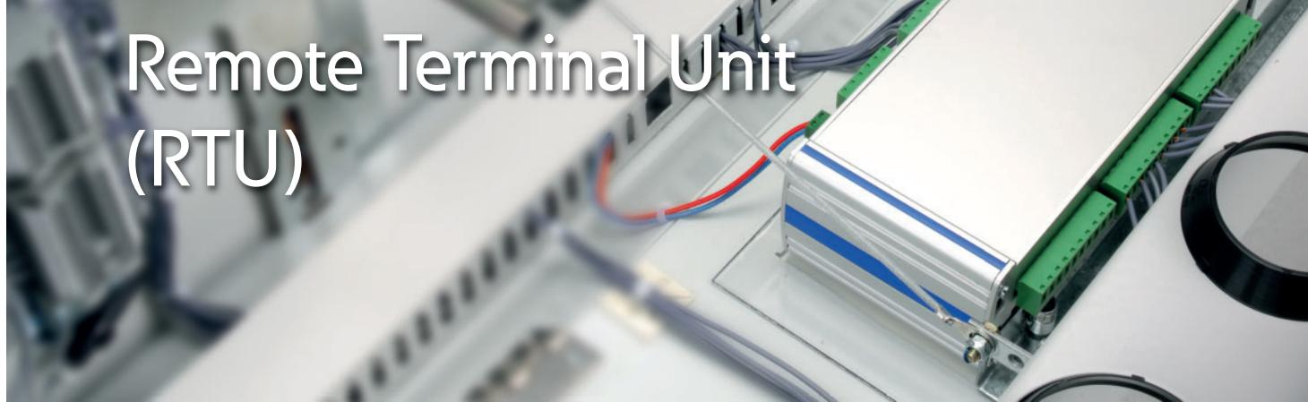
The Remote Terminal Unit is a device for acquiring, processing, storing and transmitting information
