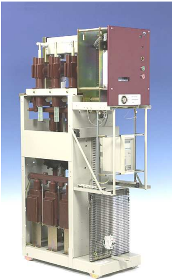
Fig.2 An example of a retrofit solution: The minimum-oil breaker in fig.1 can be replaced by a new truck; including a modern vacuum breaker actuated by an electro-mechanical drive.
